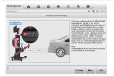
Place the calibration frame directly behind the vehicle. Follow the on-screen instructions to adjust the calibration frame.
