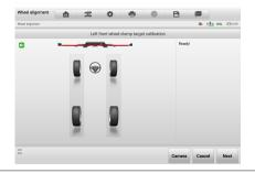
When the distance between the calibration frame and the front vehicle is in the required range (87–94 inches), the centers of the calibration frame and the vehicle are aligned, and the crossbar is adjusted to the required height, tap **Next**. Then the tablet will indicate that everything is ready for the next step.
