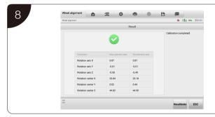
After collecting data, the tablet will display the calibration result automatically. If the screen displays  $\bigcirc$ , it indicates that the calibration is successful. You can tap **ESC** to exit the function. If the screen displays  $\bigcirc$ , it indicates the calibration has failed. You need to tap **Recalibrate** to perform the calibration again.
