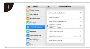
Tap Maintenance & Service on the ADAS & Aligner Settings screen, then select Accuracy Check on the right of the screen.
