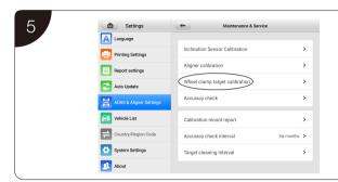
After selecting the clamp type, tap the **Back** button to return to the ADAS & Aligner Settings screen. Tap **Maintenance & Service** on the ADAS & Aligner Settings screen, then select **Wheel Clamp Target Calibration**.
