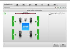
Push the vehicle as shown in the on-screen instructions (Forward — Backward — Forward) to perform the wheel rolling compensation test. Wait for the tablet to automatically advance to the next screen.
